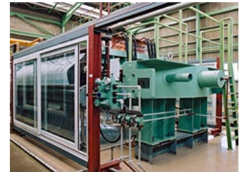
Ion-exchange membrane process for chlor-alkali electrolysis
